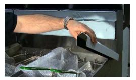
Figure 7. Install joiner strip(s) after fryers are connected.
